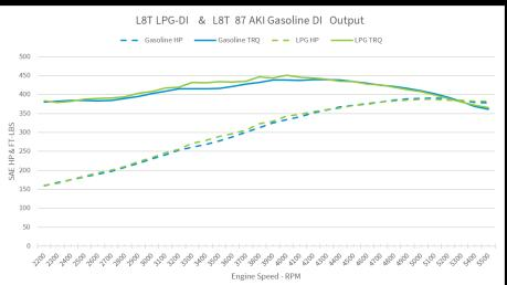
Using direct injection avoids the 20 percent power reduction associated with port fuel injection
